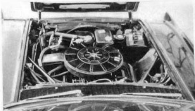
AIR CLEANER and accessories effectively conceal Lincoln's 430cu.in. V8 engine which provides good acceleration and 110-plus m.p.h. top speed.
