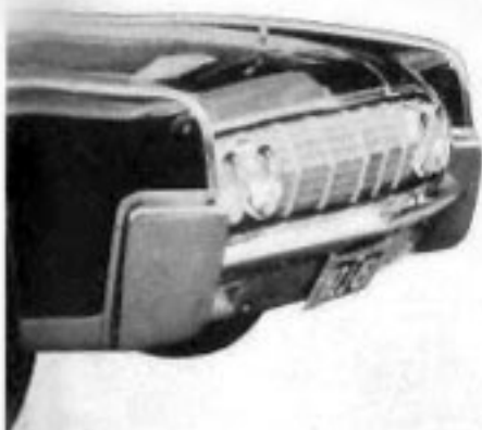
AIR CLEANER and accessories effectively conceal Lincoln's 430cu.in. V8 engine which provides good acceleration and 110-plus m.p.h. top speed.
