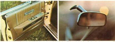
Door panels are beautifully appointed and finished to complement the interior decor. Walnut-grained vinyl paneling is optional at no extra cost. The rear view mirror is bonded to the windshield, ideally located for improved visibility and easy adjustment. Its shorter bracket arm minimizes vibration.
