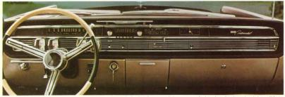
The control panel is redesigned for greater convenience, into a single gleaming sweep. It incorporates the four duets for the optional air conditioner. These duets are spaced along the control panel and are individually adjustable so that air flow can be distributed evenly and gently through the car.
