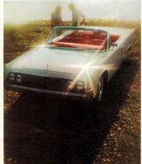
There is a lifetime of gleaming beauty in this lustrous enamel finish. The Continental body is protected by three coats of acrylic enamel, baked onto it over two protective primer coats. The color lasts with the car.
