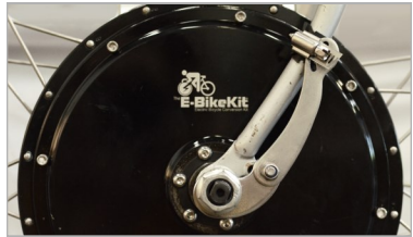
Connect the arm to axle and frame
