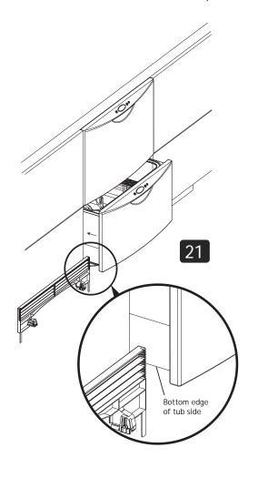
Partially open the bottom drawer. Turn Prefinished Toe Kick upside down and hold vertically against the bottom edge of the *Tub side* (not the drawer front).
