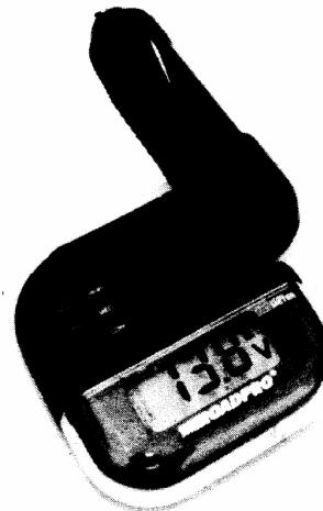
**E. CHARGING SYSTEM (ALTERNATOR & REGULATOR) OKAY?** You can check it with the voltage meter.
