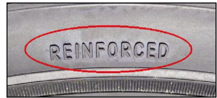
Figure 1. “Reinforced” marking on sidewall.
